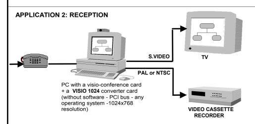
The VISIO 1024 scan converter card allows to display on a TV screen or to record on a video tape a Visio-conference communication.
