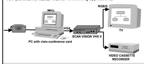
The ANALOG WAY scan converter SCAN VISION VHX II, allows to convert all computer signals from PC or MAC to TVs (with a RGB/S connection for a maximum quality) and to record a visio-conference communication on a videotape (VHS, S-VHS, Hi-8).
